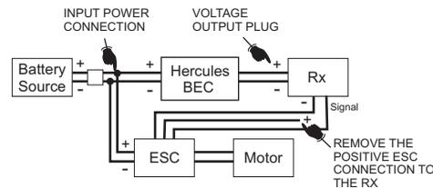
2. Plug the Hercules voltage output plug into the battery slot of the receiver. Make sure the polarity is matching with the receiver slot before inserting the Hercules plug - **black wire negative (-) and red wire positive (+)**. Connect the ESC signal connection to Rx with the positive red wire removed.
